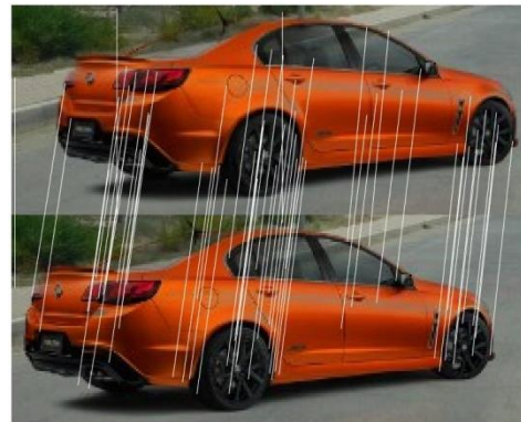
Figure 6. SIFT matching between test and reference image
