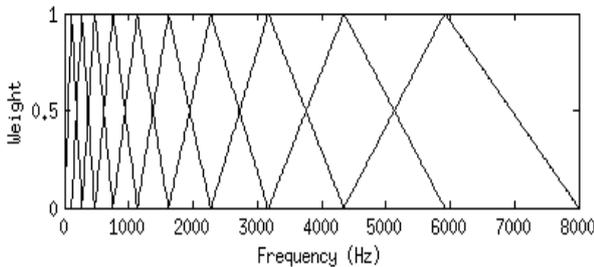
Figure 1. Mel filterbank with 10 triangular-shaped filters.
