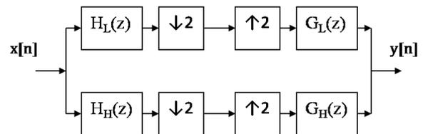
Figure 1. Two channel filter bank
