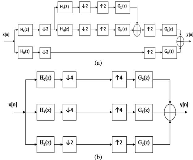
Figure 5. (a) Three-Band octave filter bank (b) Equivalent structure of three-band octave filter bank
