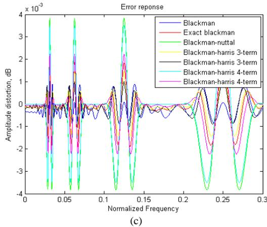
Figure 7. (a) Magnitude responses of prototype filters (b) Magnitude response of five analysis filters for Blackman window (c) Amplitude distortion for different window functions for five-band
