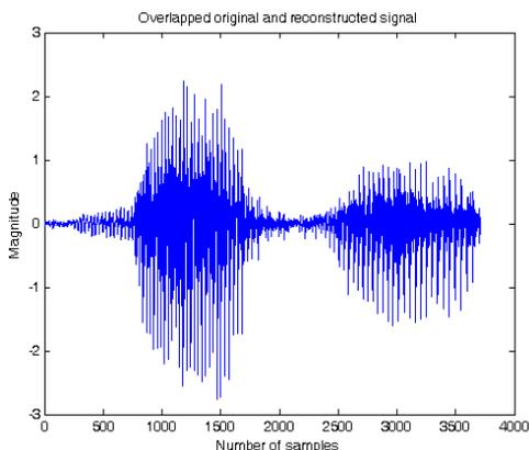
Figure 4. Overlapped original and reconstructed speech signal
