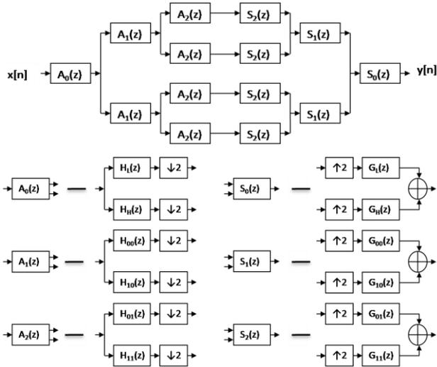
Figure 2(a). Eight-Band uniform tree-structured filter bank
