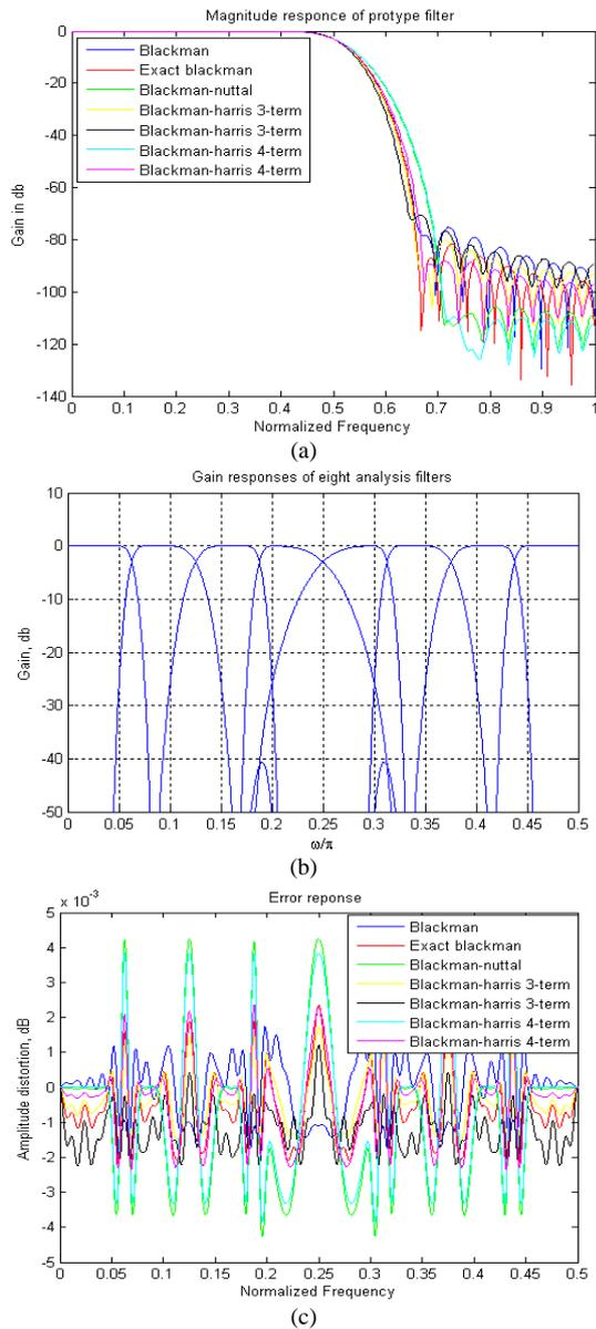
Figure 3. (a) Magnitude responses of prototype filters (b) Magnitude response of analysis filters for Blackman window (c) Amplitude distortion for different windows
