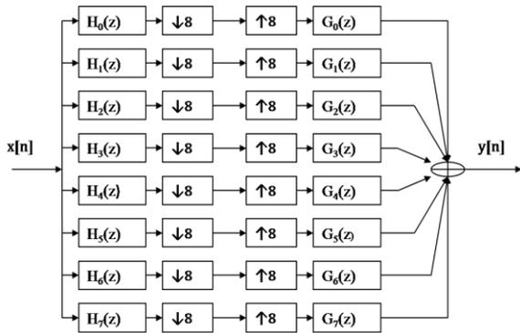
Figure 2(b). An equivalent representation of eight-band uniform tree-structured filter bank
