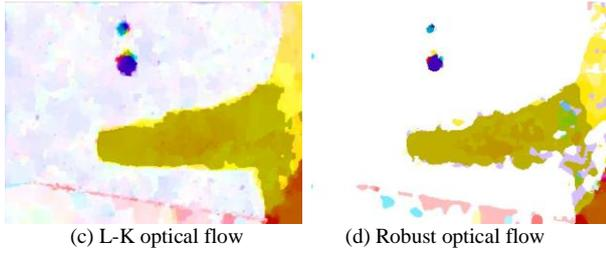
Figure 2. (a) and (b) are two frames from a noisy video, in this video, the background is steady, (c) is the robust optical flow between them, the background should be white as there is no movement, but the movement of the foreground caused the error in the background, especially the area under the arm, we call this “leak” (d) is the verified robust optical flow, in which the “leak” is suppressed
