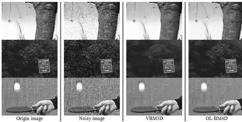
Figure 5. Visual comparison of the sequences, from top to bottom, flower garden, bus and tennis corrupted by white Gaussian noise with standard deviation  $\sigma = 20$ , denoised by the proposed algorithm OL-BM4D and the VBM3D algorithm. Our method clearly provides better result and recovers more detail
