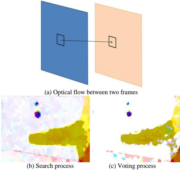
Figure 3. Verification method: (a) shows origin robust optical flow without verification between two frames. In (b), around the patch in frame b the optical flow points to, a search window is formed. In this window we search for a patch which is the most similar to the patch in frame a. As patches overlap with each other, in (c) all the patches with a particular pixel vote for the accurate optical flow of this pixel to reduce noise
