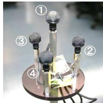
Figure 1. Tetrahedron microphone array
