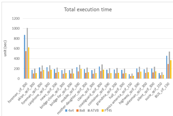
Figure 12. The execution time of encoder with 4x4, 8x8 ATVB, and proposal PT4S, respectively.
