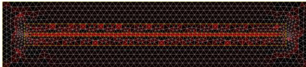
Figure 2. Schematic mesh of simulation model consisting of 20150 elements.
