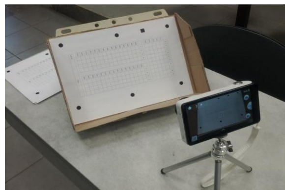
Figure 1. The setup for fast acquisition of answer sheet images.
