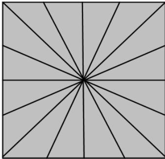
Figure 3. wedge shaped frequency partitioning with  $2^l$  directional sub bands ( $l=3$ )
