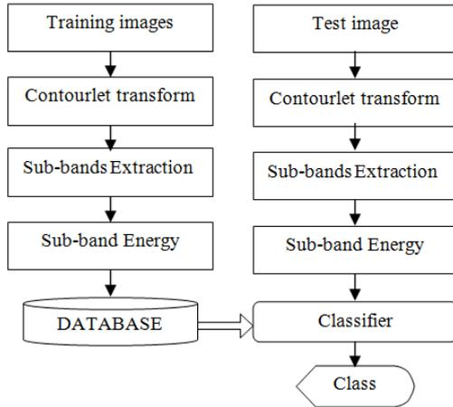
Figure. 5. Block diagram of proposed human emotion recognition system
