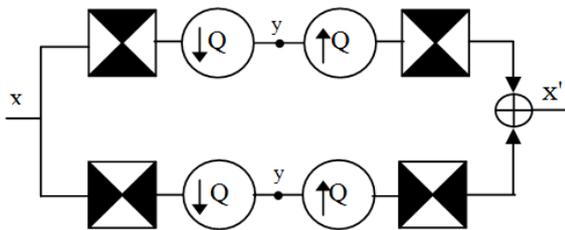
Figure 4. 2D dimensional spectrum partition using quincunx filter banks with fan filter
